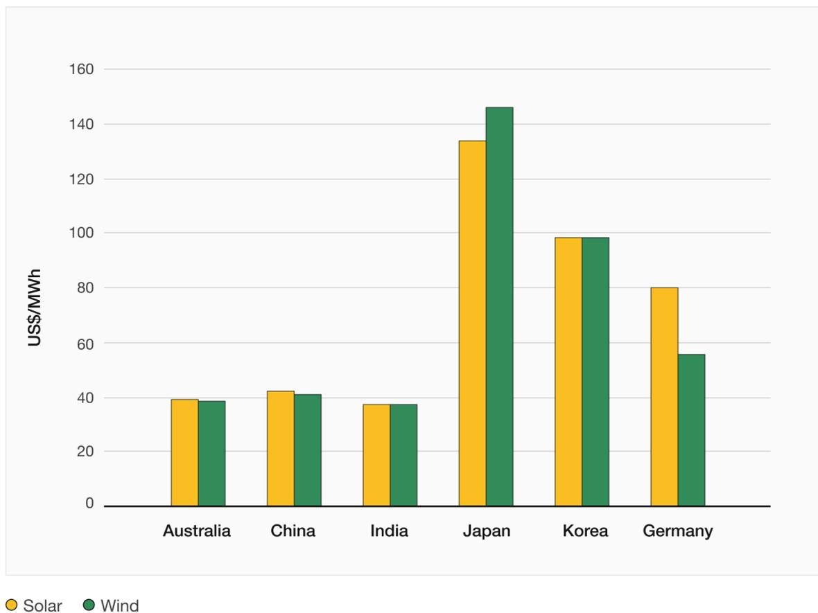
**Figure 7.1. Levelised cost of solar and wind in Australia and the five selected countries (average of IEA, 2020b, and IRENA, 2023a, 2023b)**
