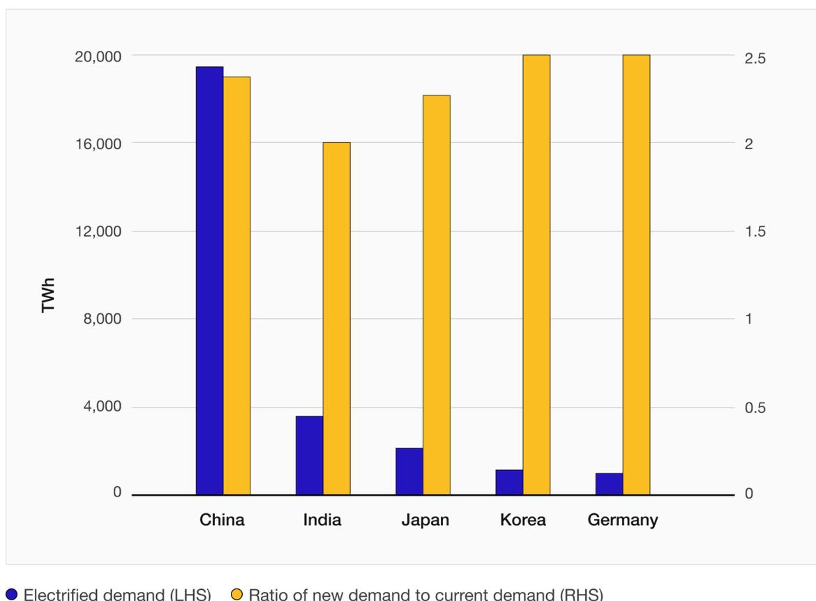
**Figure 3.4. Crude TWh required for electrification of 2021 economies, assuming full electrification with a 60 percent decline in primary energy requirements.**
