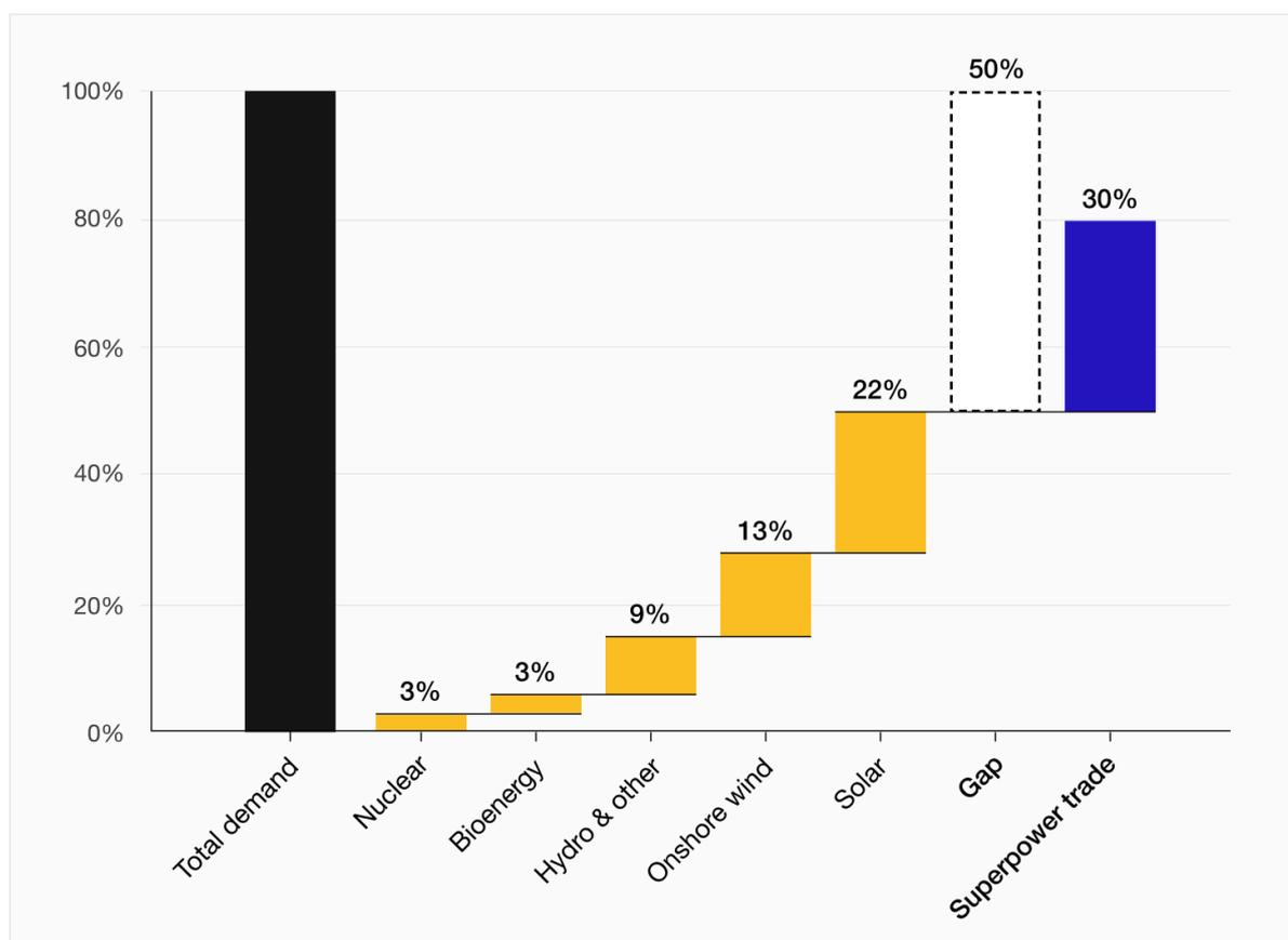
**Figure 8.1. China’s clean energy deployment based on recent trends as a share of electricity demand in 2060, the remaining supply-demand gap in 2060, and the potential contribution of the superpower trade.**
